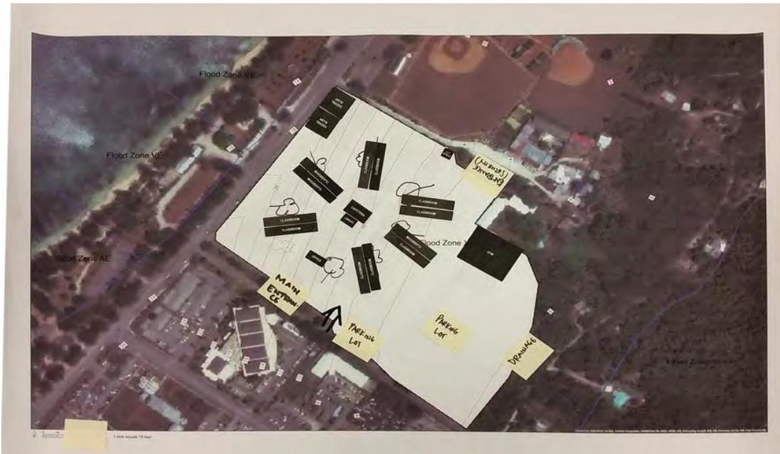
Figure 2-10 – This Centralized campus locates the Cafeteria/Library at the heart of campus, with Classroom buildings radiating outward. Parking and drainage facilities are located at the lowest/flat portion of the site.
